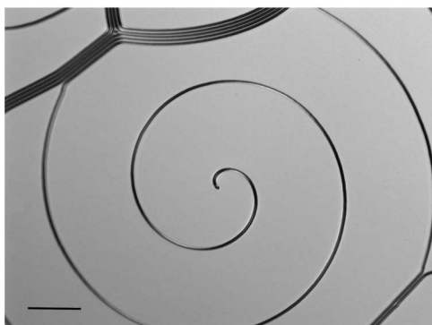
Figure 5. CF1 spiral observed in the coexistence region. Polariser and analyser are at 45^\circ degrees relative to each other. The black scale bar is 100 \mu\text{m} long. Here d = 15 \mu\text{m} , \Delta T = 40^\circ\text{C} , T = 54.5^\circ\text{C} , f = 100 \text{ Hz} .
